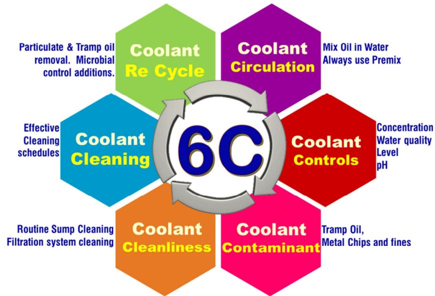
The 6C, as a concept is presented here is to demonstrate how to institutionalize a coolant management system that will effectively increase coolant life to its designed life expectancy levels thereby reducing consumption, and improving performance of the machine tool in terms of tool life, component finish, machine down time, and finally reducing disposal costs.
